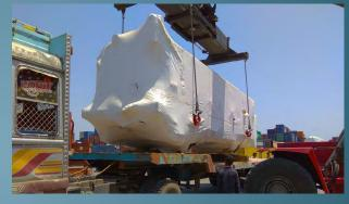
heaviest package loaded on Flat Rack weighed 67 MT.
